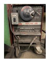
CONSTANT CURRENT AC/DC ARC WELDER MODEL AC/DC 250
